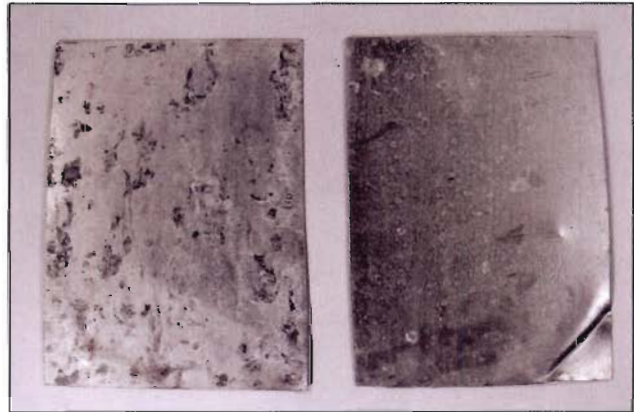
Fig.11 – samples 1 and 3 Alluminium after 360 hours
