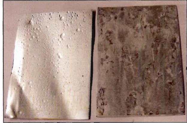
Fig.9 – samples 2 and 3 Alluminium after 192 hours
