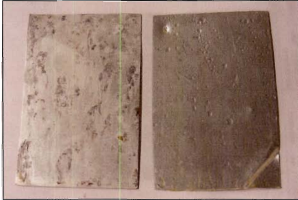
Fig.8 – samples 1 and 3 Alluminium after 192 hours
